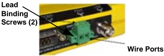
Figure 2. Power Connector Polarity: Left +, Right –
