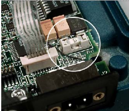
Figure 16. Internal Fuse and Holder Assembly Location
